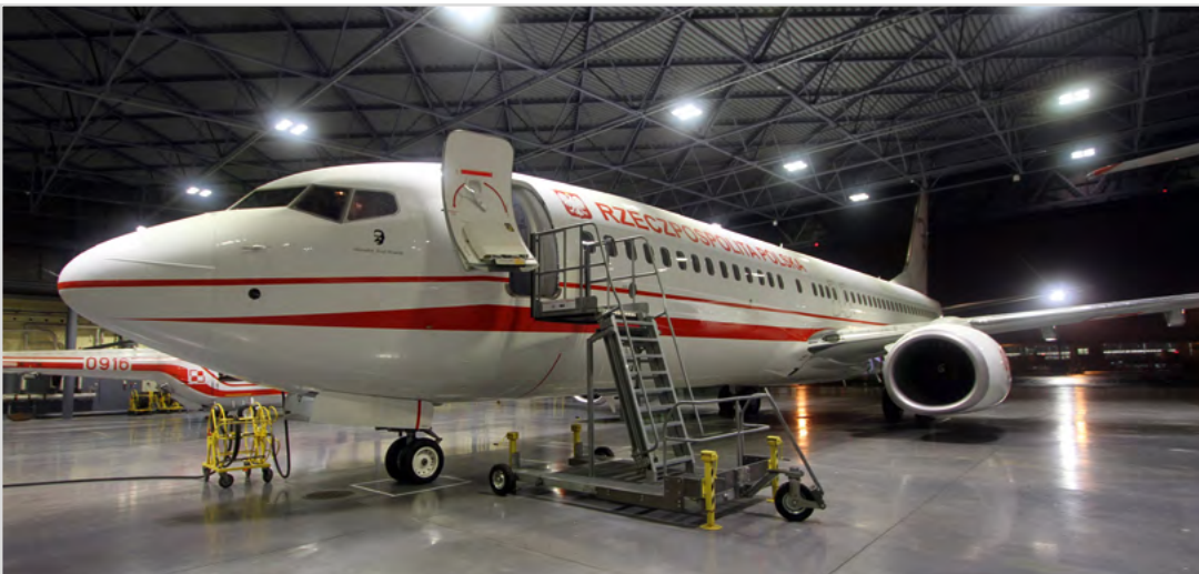
❷ Service platform - another device manufactured by WCBKT S.A., enabling ground support for aircrafts such as Boeing 737.
