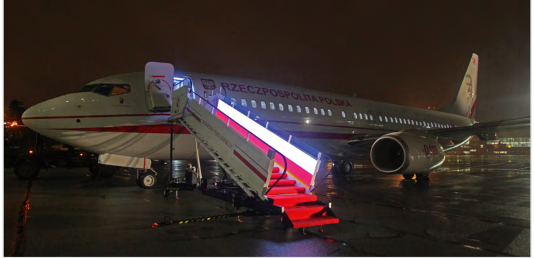
❶ A special version of the LSP 3S passenger stairs for the support of a government Boeing 737-800 aircraft.
