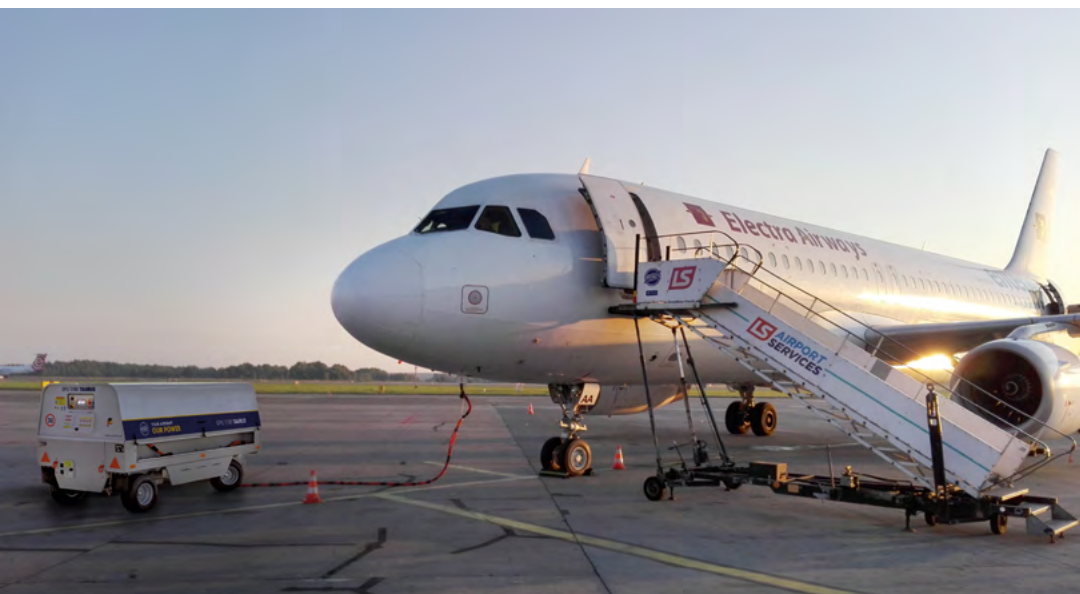
GSE equipment (GPU-7/90 Taurus power supply unit and LSP3S passenger stairs) produced by WCBKT S.A. Photo: WCBKT S.A.
