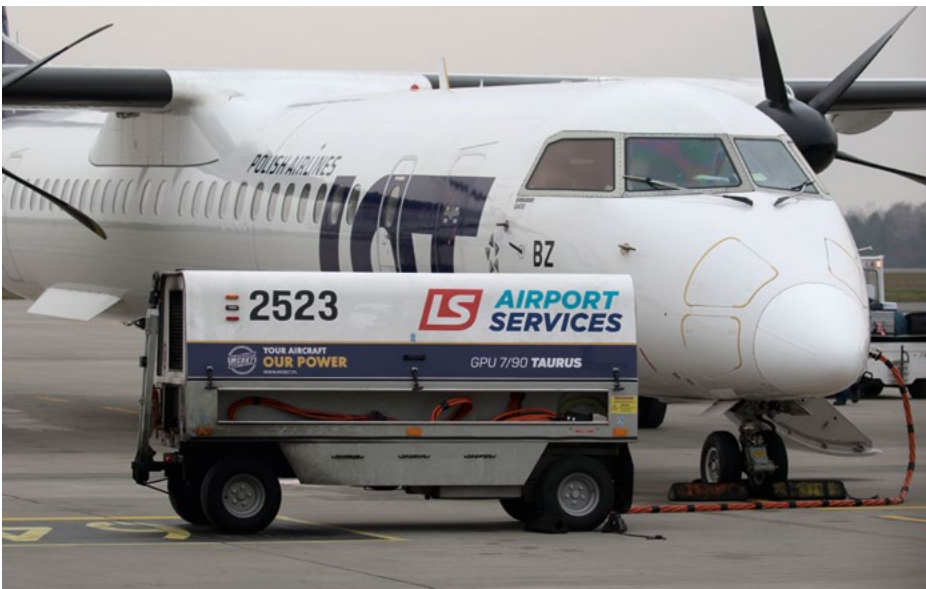
GPU 7/90 TAURUS powering Bombardier Q400 at Chopin Airport in Warsaw. Photo: Jakub Bytner.
